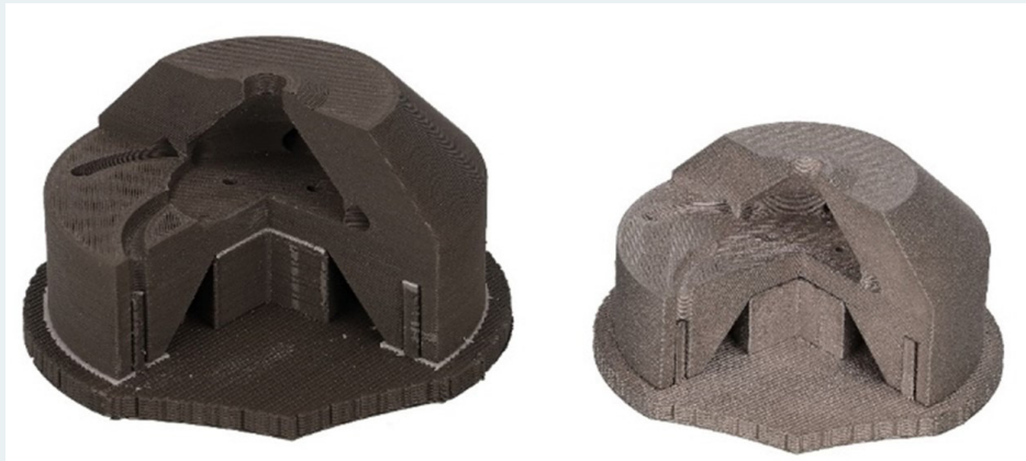
Figure 1 Green part with support structures and Ultrafuse Support Layer and sintered part with support structure
