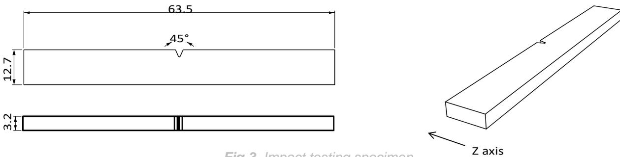
Fig 3. Impact testing specimen
