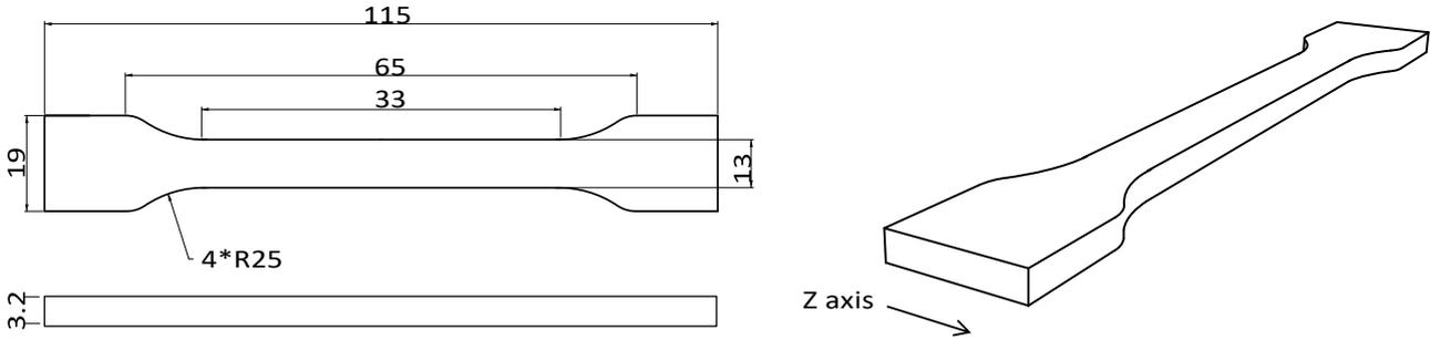
Fig 1. Tensile testing specimen
