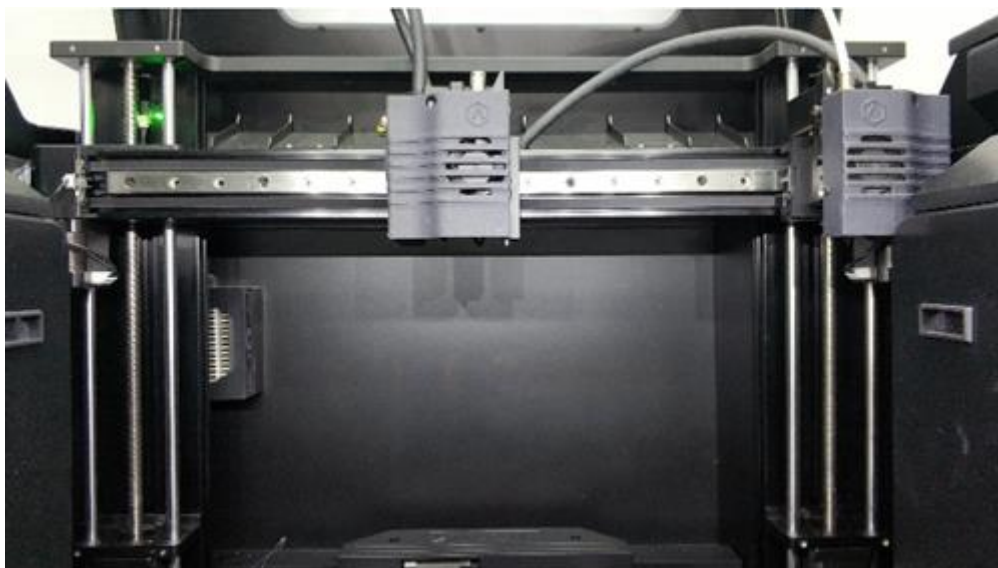
Figure 3 Disable the motor and move the extruder to the center.
