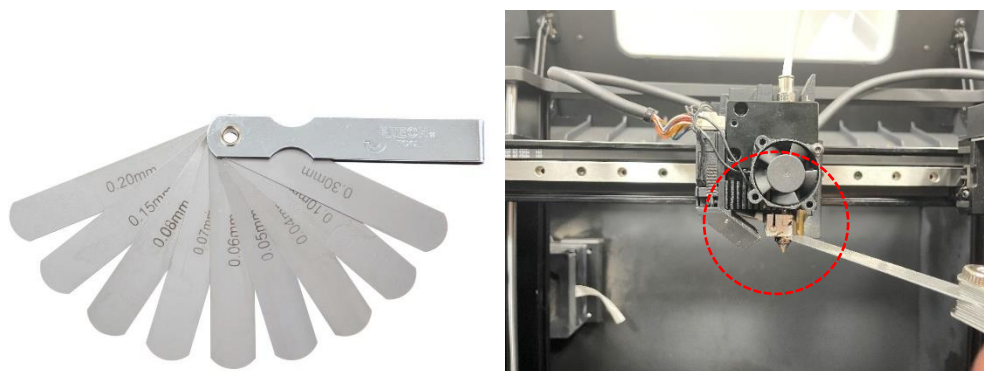
Figure 10 Check the spacing between the nozzle and the heater block with a feeler gauge.
